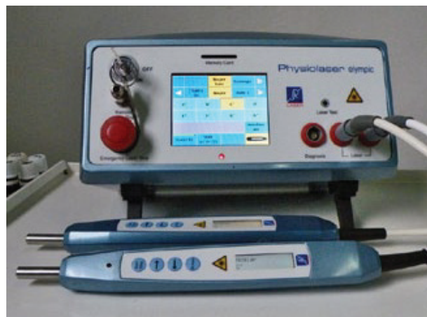
Figure 3: Physiolaser (2x 90 Watt, 904nm, impulse lasers), Reimers & Janssen, Berlin. Germany.
