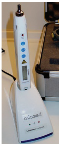
Figure 1: Laserpen (70 mW, 785 nm, cw laser), Reimers & Janssen, Berlin, Germany.
