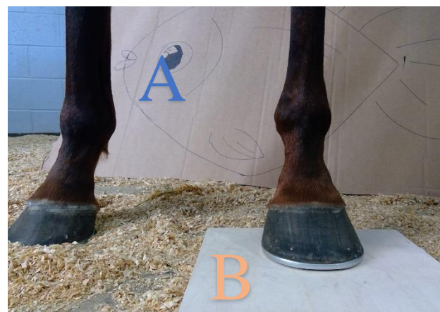
Figure 1: Before hoof images were taken, the foot was placed on a wood board (B). To ensure that nothing was in the frame that would increase camera temperature range, a cardboard screen (A) was used to block the rear legs of the horse and other objects in the stall.
